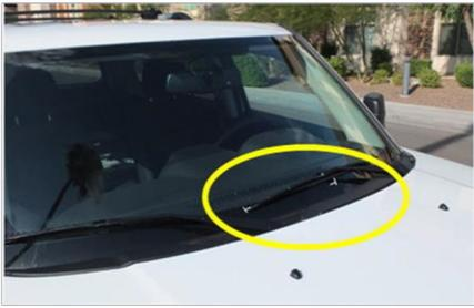
Figure – 1: Lining up of blades with T-marks for correct location of blade during assembly process.
